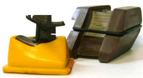
Fluroelastomer & Dacron® Prototype Bladder
