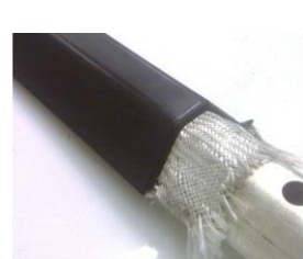
Fluroelastomer & Dacron® Prototype Bladder
