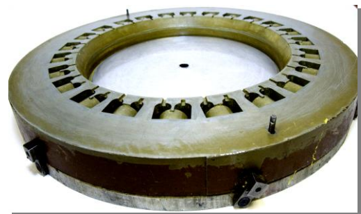
Epoxy and Alloy Spin Cast Mold produces Urethane Vibration Dampeners
